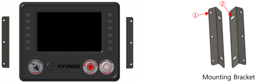
[Fig. 2-4] Flush Mounting Type Diagram
