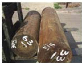
Lignumvitae (for Domestic Model) (Hard Wood from South America Coated with Paraffin)
