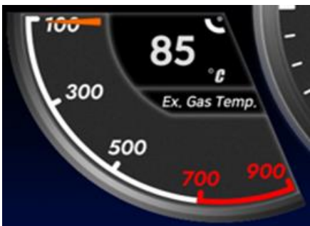
[Fig. 3-24] Exhaust Gas Temperature
