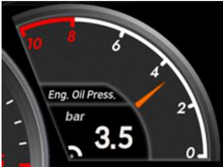
[Fig. 3-23] Engine Oil Pressure Gauge
