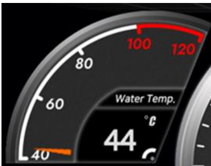
[Fig. 3-19] Engine Cooling Water Temperature
