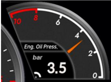
[Fig. 3-20] Engine Oil Pressure Gauge
