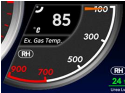
[Fig. 3-26] Exhaust Gas Temperature RH
