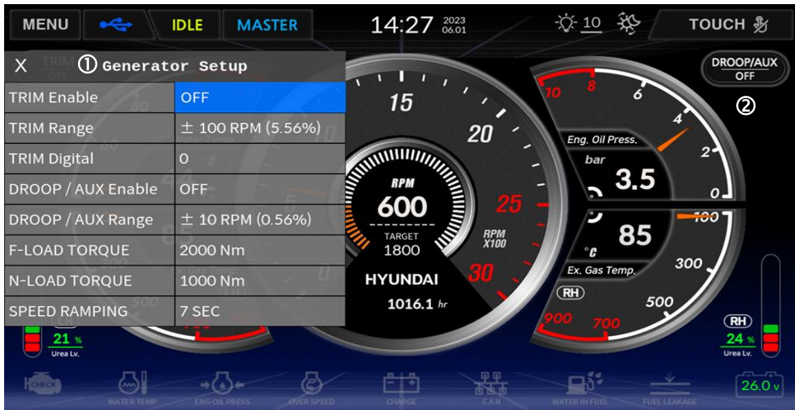
[Fig. 3-18] Generator Configuration Settings
