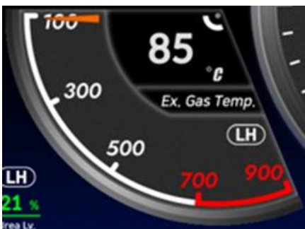
[Fig. 3-25] Exhaust Gas Temperature LH
