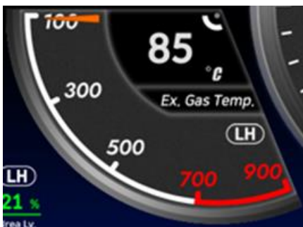
[Fig. 3-22] Exhaust Gas Temperature LH
