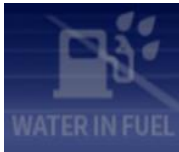
[Fig. 3-27] Water In Fuel
