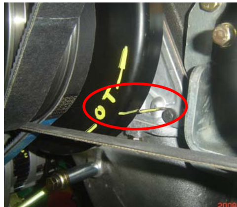
1) At "OT" position, Mark the line across damper & engine
